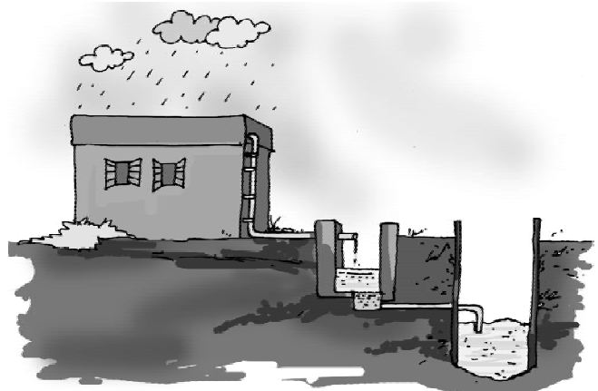
Fig. 14.13 Rooftop rainwater harvesting
