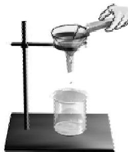
Fig. 5.10 Filtration using a filter paper
