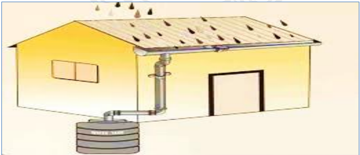
Fig. Diagram showing a model of roof-top rain water harvesting structure
