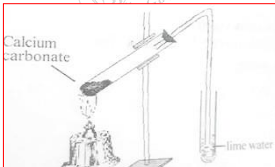
Fig. Heating of calcium carbonate and giving out carbon dioxide gas which turns lime water milky.
